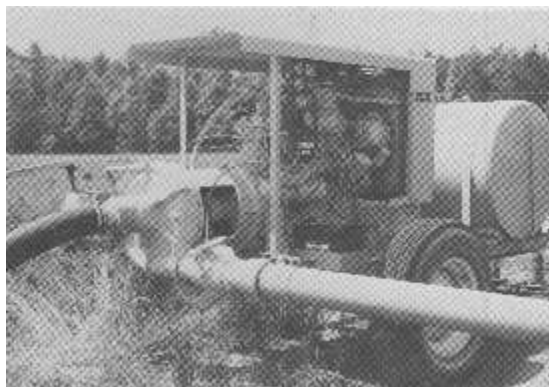
Figure 7. Close-coupled engine-driven centrifugal pump.
